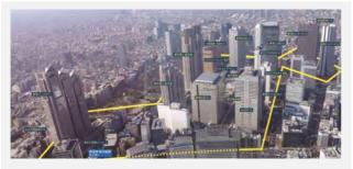
The centre has a cooling capacity of 65,000RT and is one of the largest systems in the world that accommodates more than 20 skyscrapers in the Shinjuku area. This system uses natural gas and the latest technologies such as energy regeneration towards sustainable urban environments through reduced energy consumption.
