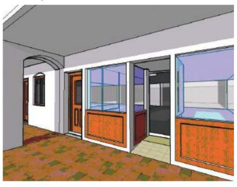
Figure 5.26 - Differences In Level Between Verandah Way And Unit To Be Taken **Up Within The Unit**
